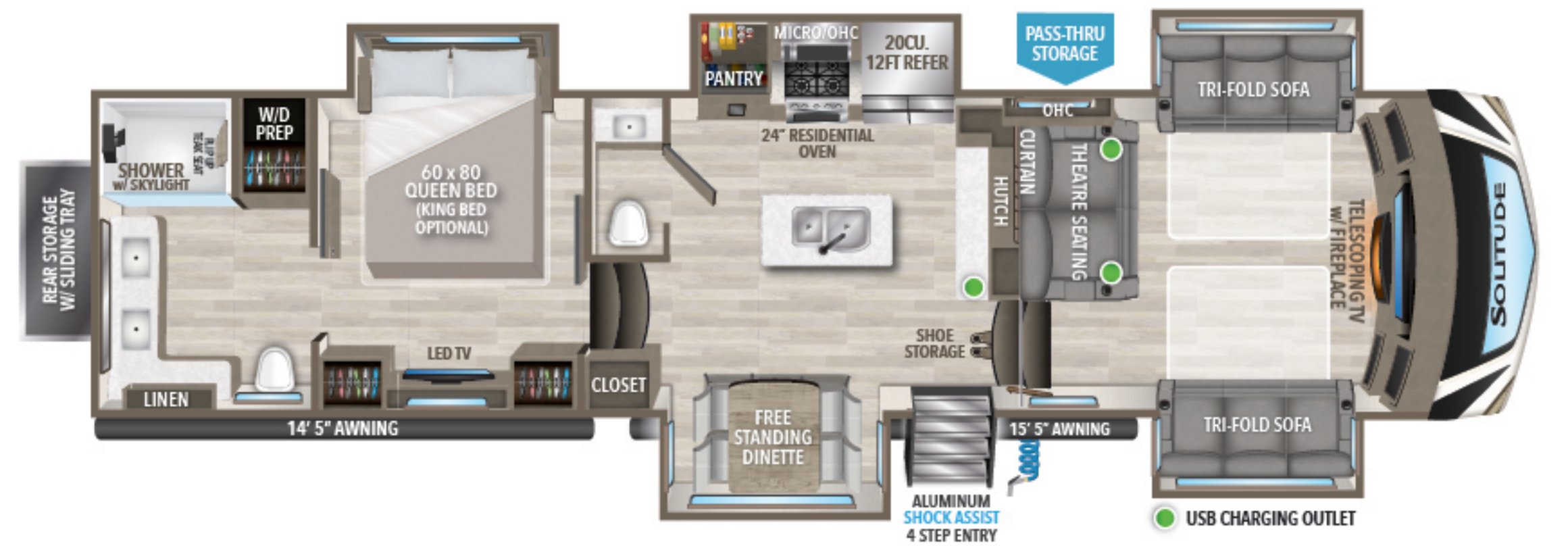
380FL UVW † 14,866 HITCH ‡ 3,052 GVWR 16,800 LENGTH ‡ 41' 5" HEIGHT 13' 5" CAPACITY 81 106 106
