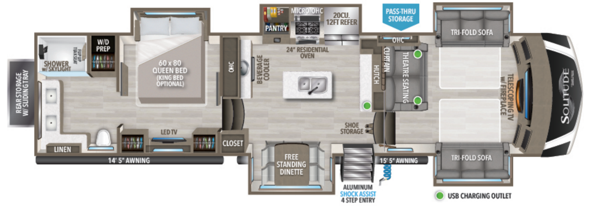
382WB UVW † 14,866 HITCH ‡ 3,052 GVWR 16,800 LENGTH ‡ 41' 5" HEIGHT 13' 5" CAPACITY 81 106 53
