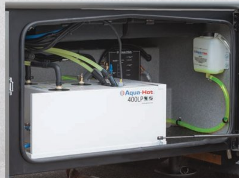
Designed and created by an RV enthusiast, our Aqua-Hot hydronic heating system provides quiet, evenly-distributed heat and unlimited hot water without the dryness created by a traditional LP furnace. It also offers utility bay heat, zoned heating, and dual power sources.
