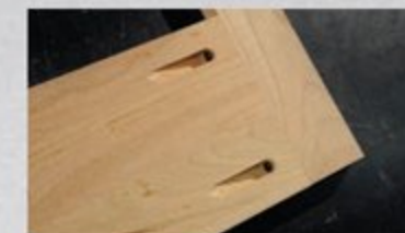
Pocket screws for structural integrity
